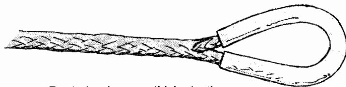
Bent aluminum or thick plastic tube spliced into towline loop
